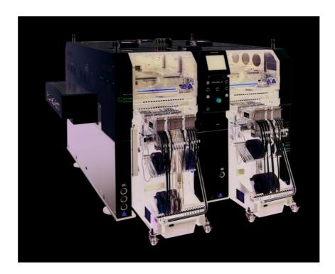
High placement quality and high throughput are the characteristics of Panasonic's NPM-DX, the next generation of smart pick and place equipment.
