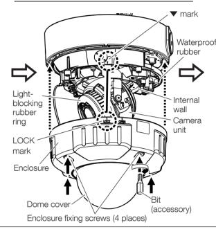
\* There is a ventilation opening inside the enclosure. Do not caulk (fill the clearance between the enclosure and the ceiling or wall with sealants or other materials) as
