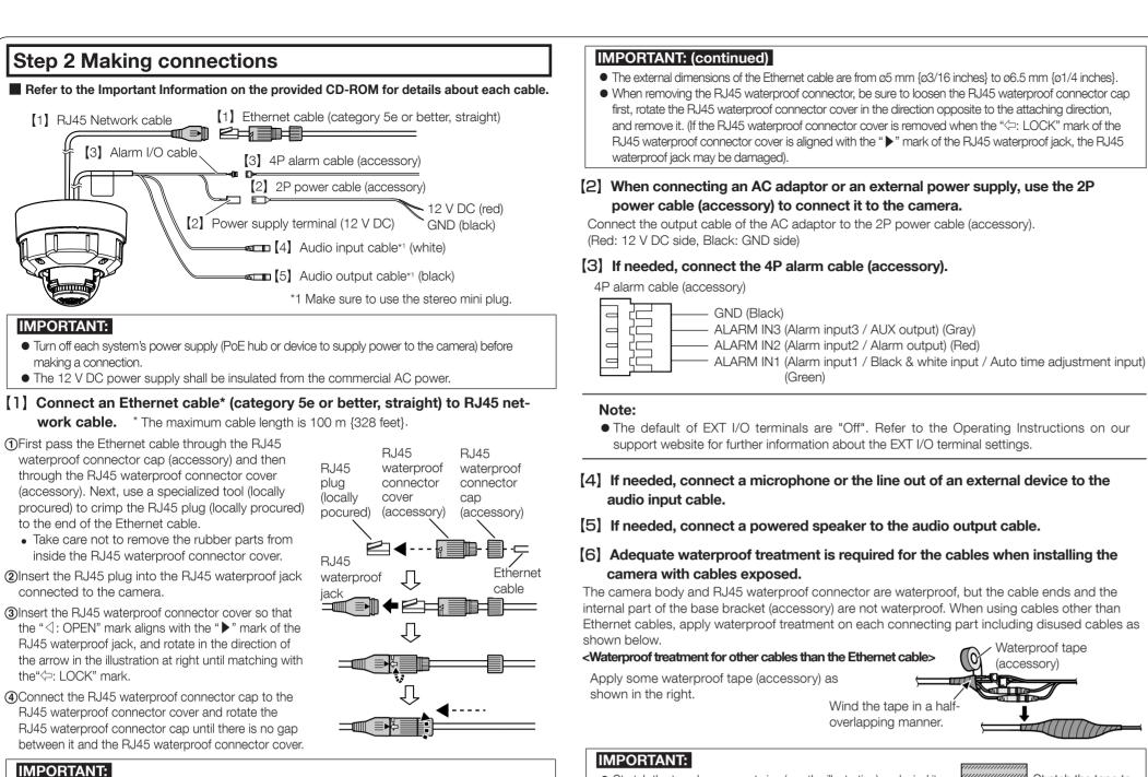
• If the procedure for the RJ45 waterproof connector (accessory) part is not correctly followed, the
