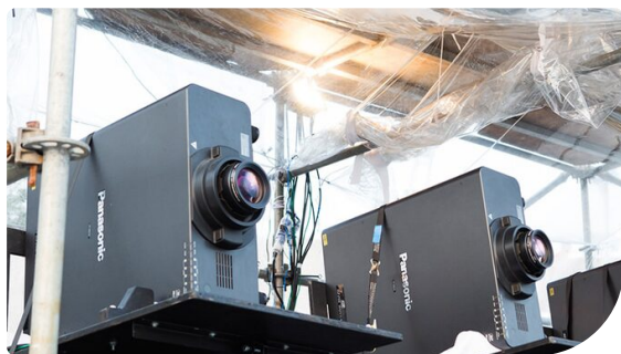
Portrait mode capability enabled projection onto long, vertical screens with a minimal number of projectors.
